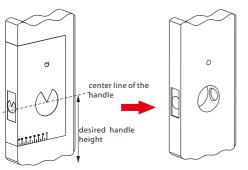
**Note 1:** Align the template along the vertical center line of the latch(D) at the desired handle height, and tape it to the door.
